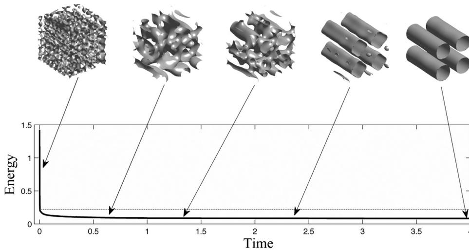
FIG. 12. *Typical energy decay.  $\Omega = [-\pi/4, \pi/4]^3$ ,  $\varepsilon = .04$ ,  $\gamma = 25$ , and  $m = 0.35$ . It is important to note that while the solution changed significantly over the entire time interval, the energy hardly changed at all after an initial transient.*
