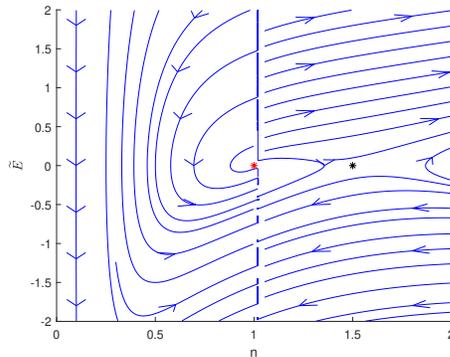
FIG. 6. Phase plane of  $(n, \tilde{E})$  with  $\alpha = 2$ ,  $b = 1.5$ , and  $J = 1$  in the case of a subsonic doping profile. The red  $*$  is the singular point  $(1, 0)$ ; the black  $*$  is the stable point  $(1.5, 0)$ .
