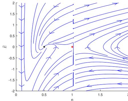
FIG. 2. Phase plane of  $(n, \tilde{E})$  with  $\alpha = 1$ ,  $b = 0.5$ , and  $J = 1$  in the case of a supersonic doping profile. The red \* is the singular point  $(1, 0)$ ; the black \* is the stable point  $(0.5, 0)$ .
