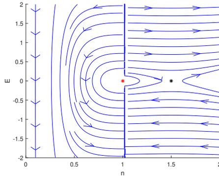
FIG. 5. Phase plane of  $(n, E)$  with  $\alpha = 0$ ,  $b = 1.5$ , and  $J = 1$  in the case of a subsonic doping profile. The red  $*$  is the singular point  $(1, 0)$ ; the black  $*$  is the equilibrium point  $(1.5, 0)$ .
