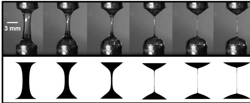
Figure 8: Comparison of the shape of the filament between CABER experiment and numerical simulation for  $x_0 = 24\%$ ,  $Ec_0 = 0.040$ ,  $P_0 = 3.1 \times 10^{-3}$ . The images are separated by a constant dimensionless time interval  $\Delta t = 2$ .
