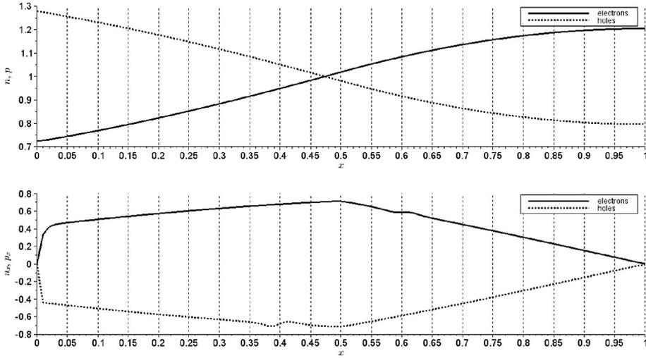
Fig. 4. Behaviour of the charge densities  $n$  and  $p$  and their first derivatives,  $n_x$  and  $p_x$ , assuming  $h = 50$ . We observe a small oscillation in the values of  $n_x$  and  $p_x$  around  $x + \delta$  and  $x - \delta$ , respectively.
