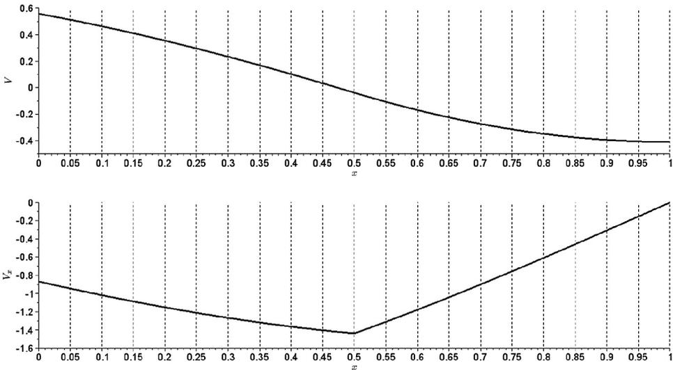
Fig. 9. Behaviour of the electrical potential  $V$  and its first derivative  $V_x$ , assuming  $h = 150$ .
