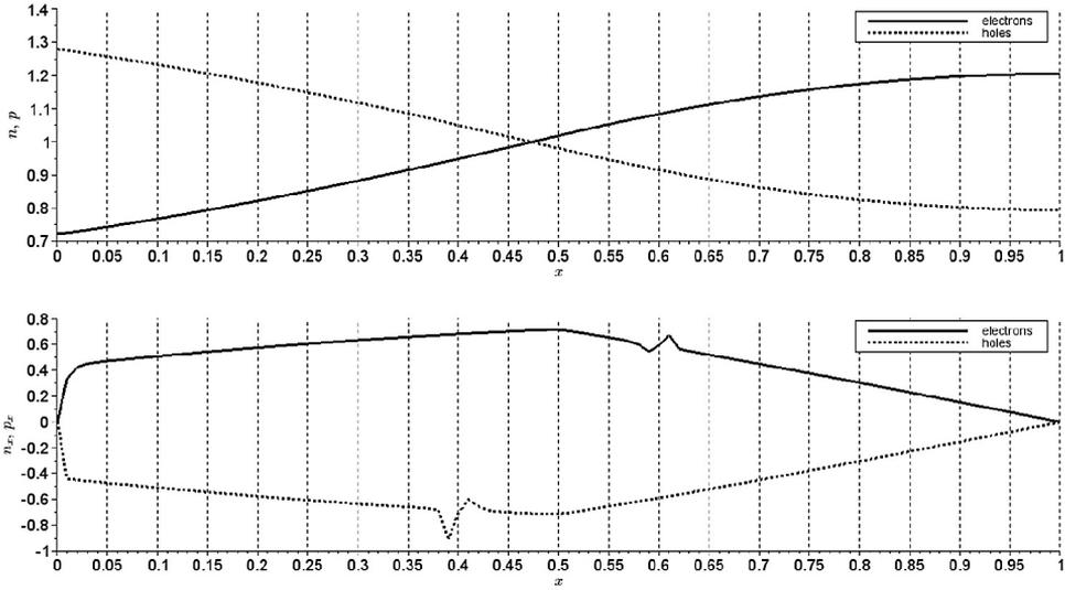
Fig. 8. Behaviour of the charge densities  $n$  and  $p$  and their first derivatives,  $n_x$  and  $p_x$ , assuming  $h = 150$ . The amplitude of the oscillations of  $n_x$  and  $p_x$  around  $x + \delta$  and  $x - \delta$ , respectively is still increasing.
