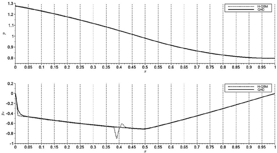
Fig. 15. Behaviour of the charge densities  $p$  and  $p_x$  computed using the H-QBM ( $\hbar = 150$ ) and the QHD. An oscillation of  $p_x$  around  $x - \delta$  is visible only for the H-QBM. This effect at the interface is a consequence of the modified Bohm potential.
