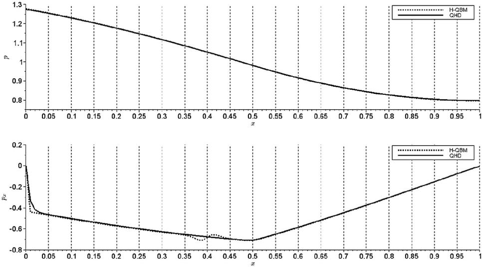
Fig. 12. Behaviour of the charge densities  $p$  and  $p_x$  computed using the H-QBM ( $h = 50$ ) and the QHD. An oscillation of  $p_x$  around  $x - \delta$  is visible only for the H-QBM. This effect at the interface is a consequence of the modified Bohm potential.
