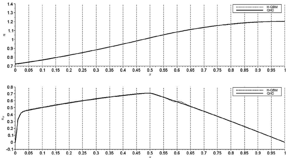
Fig. 11. Behaviour of the charge densities  $n$  and  $n_x$  computed using the H-QBM ( $h = 50$ ) and the QHD. An oscillation of  $n_x$  around  $x + \delta$  is visible only for the H-QBM. This effect at the interface is a consequence of the modified Bohm potential.
