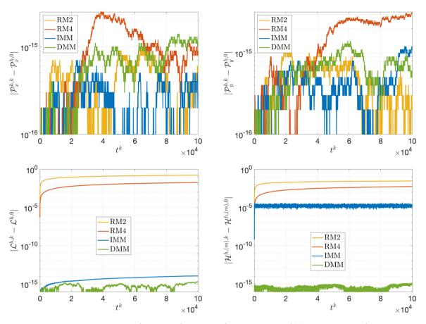
**Fig. 4.2.** Error over time in conserved quantities  $\mathcal{P}_{x}^{h}$  (top-left),  $\mathcal{P}_{y}^{h}$  (top-right),  $\mathcal{L}^{h}$  (bottom-left), and  $\mathcal{H}^{h,(m)}$  (bottom-right) for  $m^{th}$  order vortex method. Here, (13) was solved with m = 4, M = 100,  $T = 10^{5}$ , and  $\tau = 1.0$  using RM2, RM4, IMM, and DMM.
