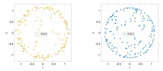
**Fig. 4.6.** Numerical path of a single vortex which is initially located at (-1 + h/2, -1 + h/2) when (13) is solved via RM2 (left), IMM (right) with T = 1650 s,  $\tau = 1.0$  and M = 25. Stars show the position of the vortex every 10 s.
