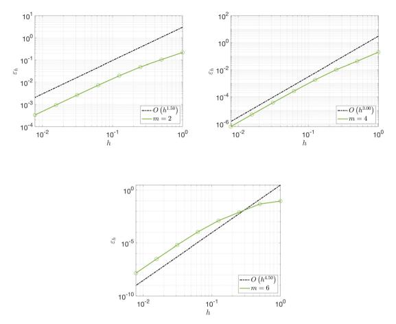
**Fig. 4.9.** Convergence of spatial error ( $\varepsilon_s$ ) to zero as the grid size (*h*) decreases when (13) is solved via (23) with m = 2, 4, 6 and T = 0.001. Each circle is a point on the convergence curve.
