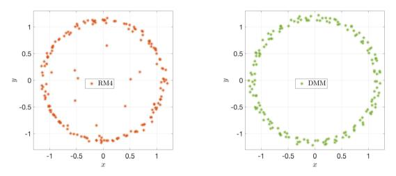
**Fig. 4.7.** Numerical path of a single vortex which is initially located at (-1 + h/2, -1 + h/2) when (13) is solved via RM4 (left) and DMM (right) with T = 1650 s,  $\tau = 1.0$  and M = 25. Stars show the position of the vortex every 10 s.
