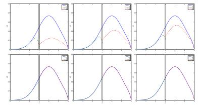
Top series of pictures shows how iterates of the Piccard-Lindeloef or classical waveform relaxation iteration converge, whilst in the the lower series by the second iteration already, iterates of the modern waveform relaxation method cannot be distinguished from the exact solution.
